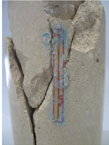
Figure 22: PL-60-11 strain gauge attached to a cylinder
