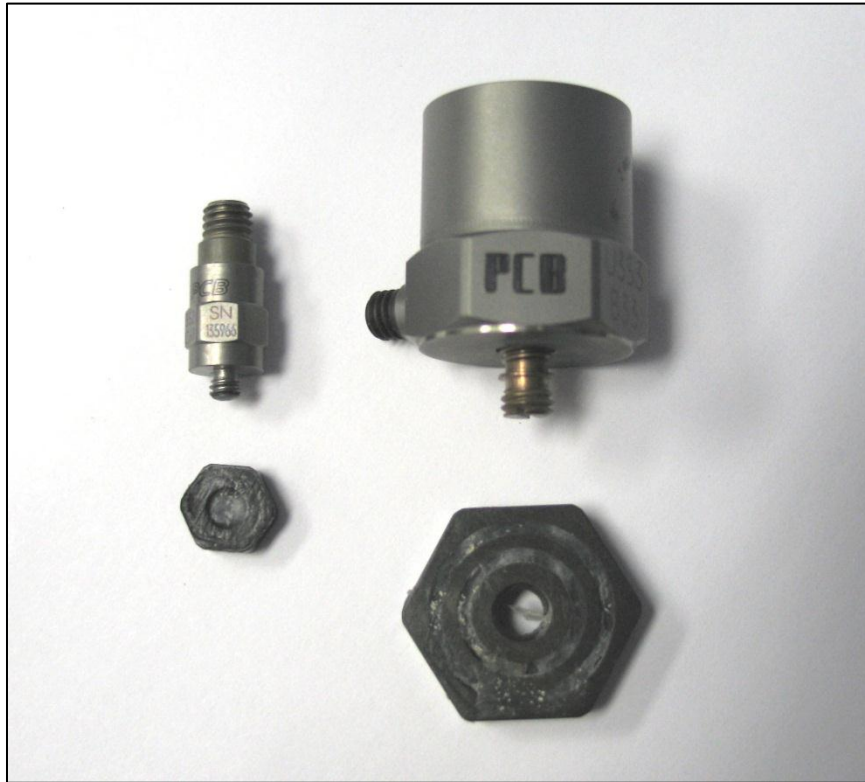
Figure 21: PCB Piezotronics Inc. adhesive mounts for accelerometer models 353B33 (right) and 352C68 (left)
