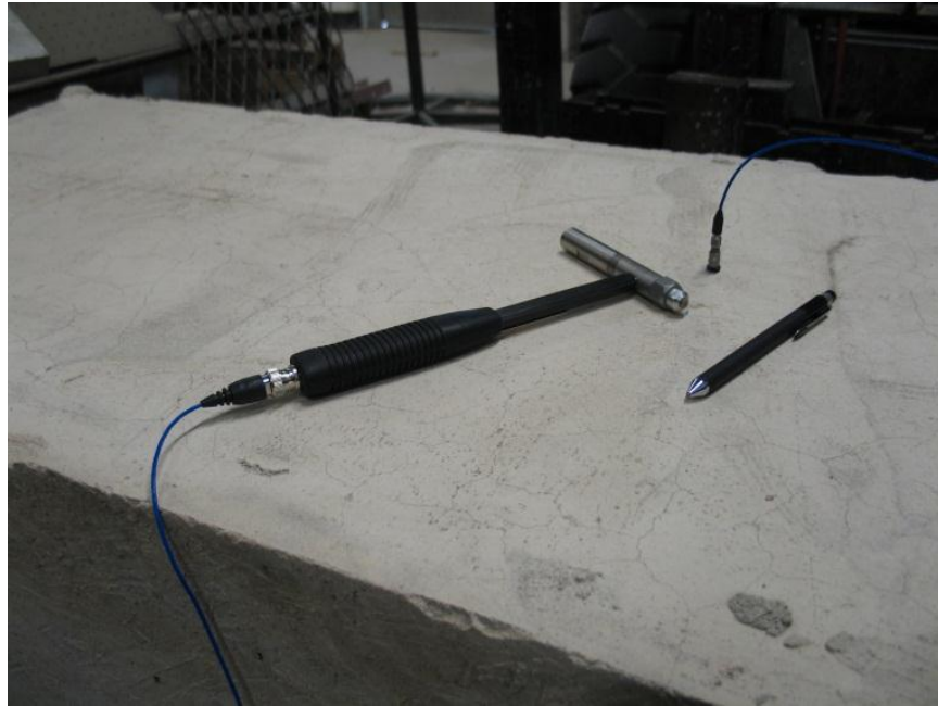
Figure 18: Impact-echo laboratory testing impact hammer and accelerometer
